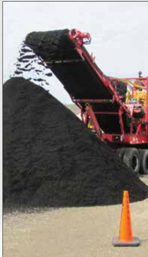
Tear-off roofing shingles being processed for use in asphalt mixture (Photo credit: LL Pelling Co.)
