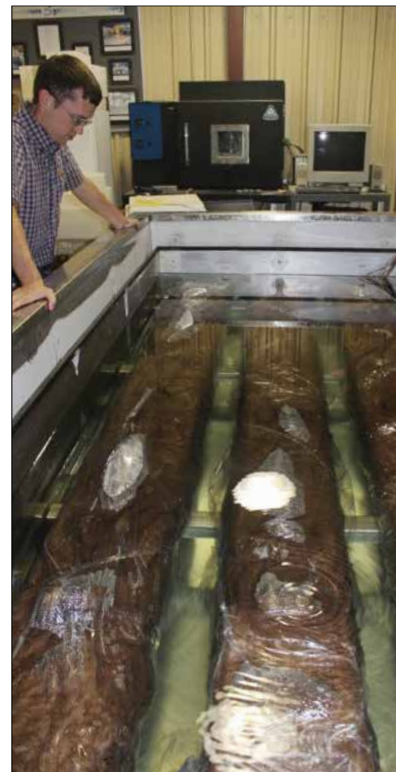
Ryan Benteman, CE research technologist, observes placement of concrete railroad ties for accelerated freeze-thaw testing at CISL.
