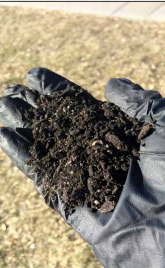
Tear-off roofing shingles are ground to have a smaller size gradation for use in asphalt mixtures.
