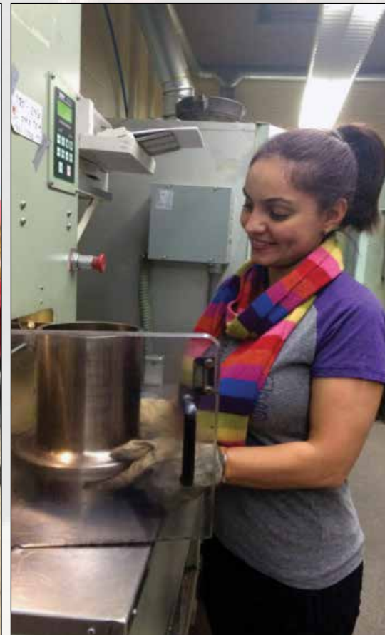
Civil engineering master's student, Masoumeh Tavakol, gets ready to compact an asphalt mixture containing RAS in the superpave gyratory compactor.
