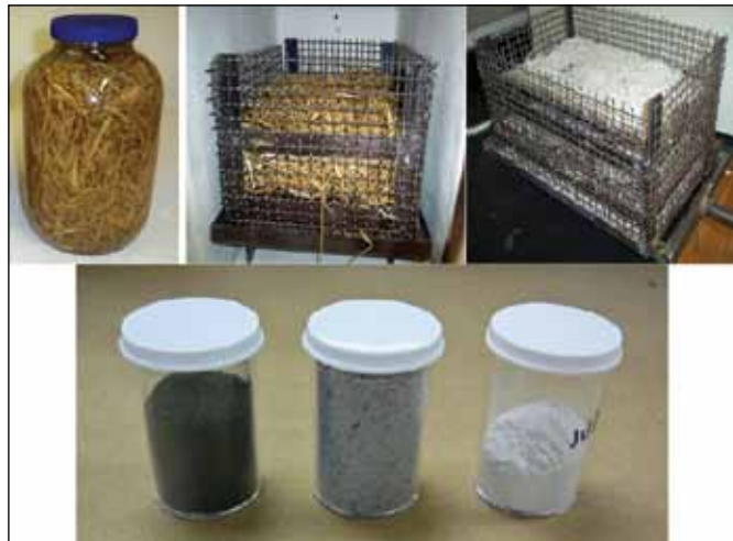
Top left: wheat straw during pretreatment; top center: straw then placed into the oven to burn and create ash; top right: ash being removed from the oven; bottom: samples of different ashes; darker ashes contain more carbon, which will compromise ash quality
