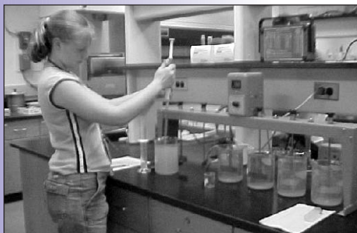
A participant at the 2003 ESSI Water Quality Workshop removes a water sample during a coagulation-flocculation experiment.
